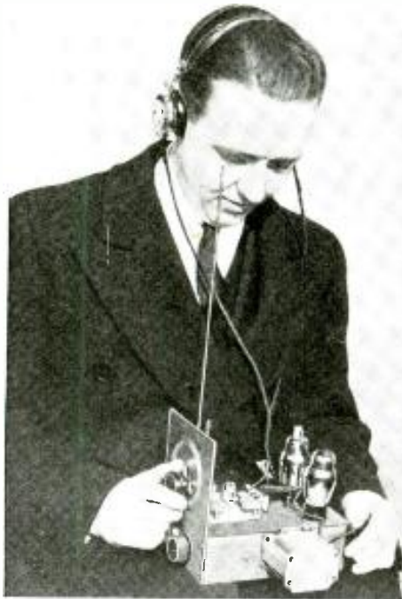
Above—The one-meter Receiver using a special super-regenerative circuit with an Acorn tube. It has a separate quenching oscillator and one stage of audio frequency amplification. The signals picked up by this receiver are fed into the main transmitter of the broadcast station.
