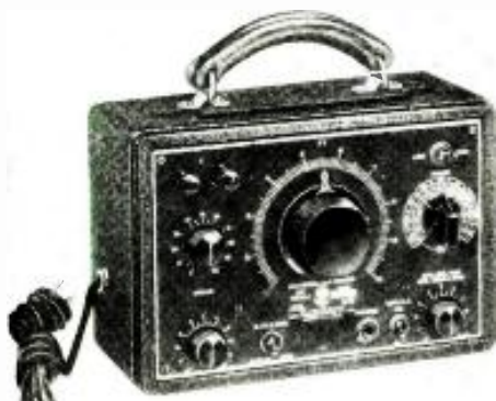
New Universal A.C. bridge which will measure capacity, resistance and inductance. (No. 541.)
