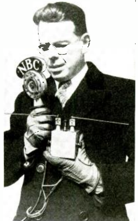
The 1-meter transmitter in use by a "foot-loose" announcer, who can move around freely—a very desirable feature at outdoor athletic games, et cetera.
