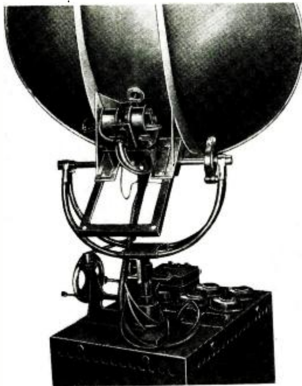
Fig. 1—Photo above shows transmitter with reflector for 3½ inch (9 cm.) waves.
